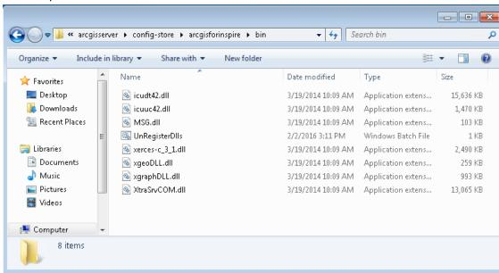
4. Open a command prompt window and run the following command regsvr32.exe /u <Path to XtraSrvCOM.dll folder>\XtraSrvCOM.dll Example:
